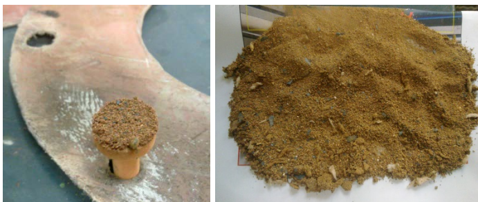
Figure 6. Basic test mode settings: UB(95)P5, 1400 \text{ }^\circ\text{C} , \lambda_1/\lambda=0.95/1.15 ; ash deposit on ceramic tablet - left, slag from reactor bottom/furnace - right
